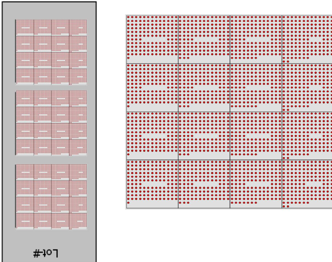
**Figure 3:** Exemplaric view for a subarray (left) consisting of 16 individual blocks. Each block (right) is calculated by number of rows vs. number of columns
