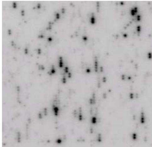
Peptide microarray was incubated with Abl kinase and [<sup>32</sup>P] ATP. Phospho-imaging on a FLA 3000 Reader was used for readout.
