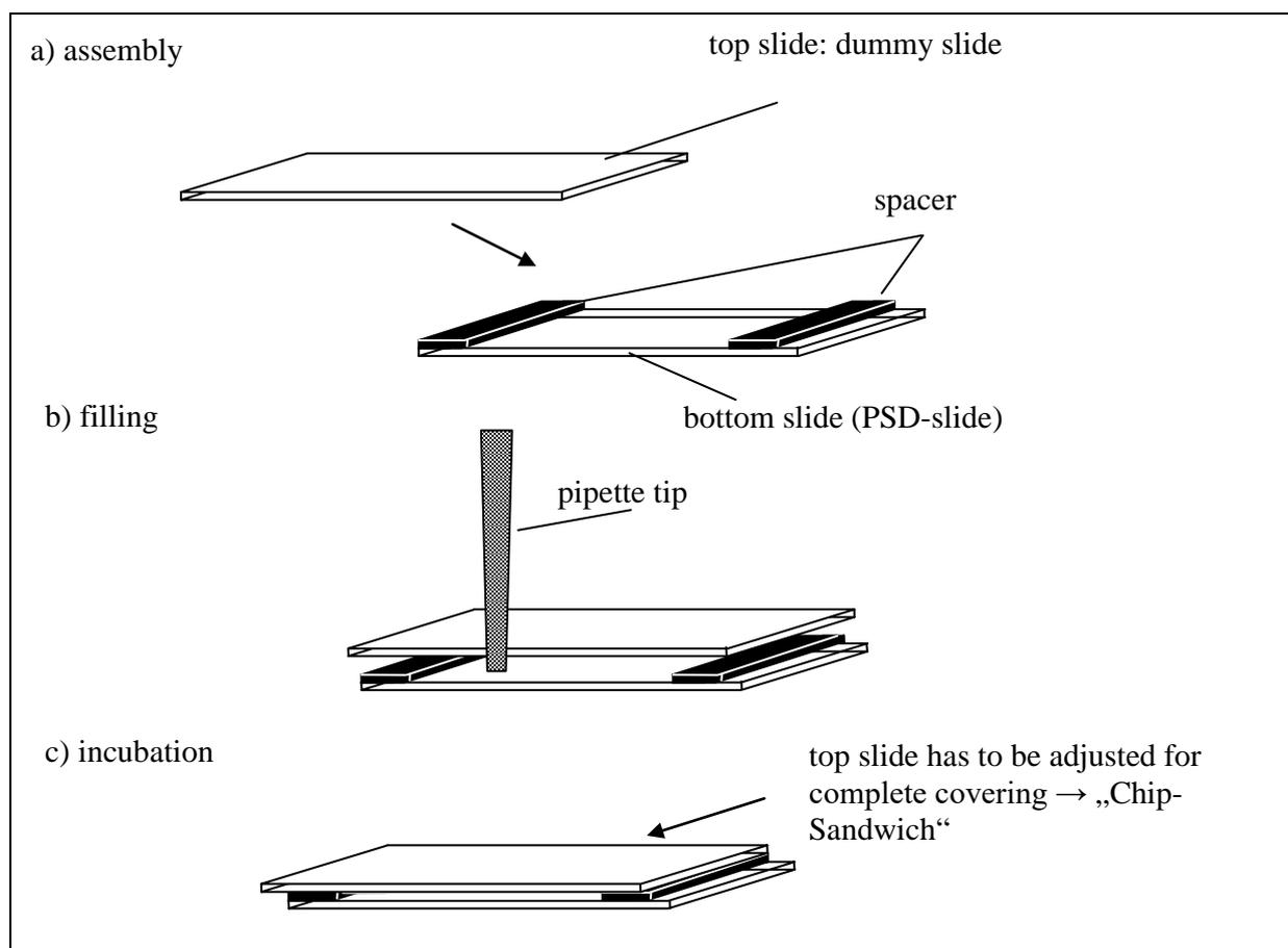
Figure 5: Assembly of "Chip-Sandwich"
